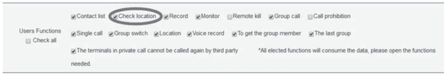
1.3 The radio should select the function for “Location” in the platform, and the radio should be outdoors to get the location. Also the programming software should be open the GPS
