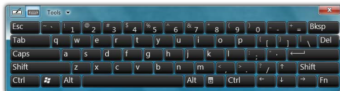
Input Panel Standard Keyboard. Can be resized to better support fingers or the stylus pen. Buttons in the upper left corner of the panel switches between on-screen keyboard and writing pad.
