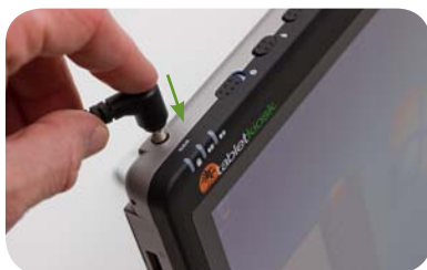
Plug the power cord into the DC Power In port on the top of the Sahara Slate PC.
