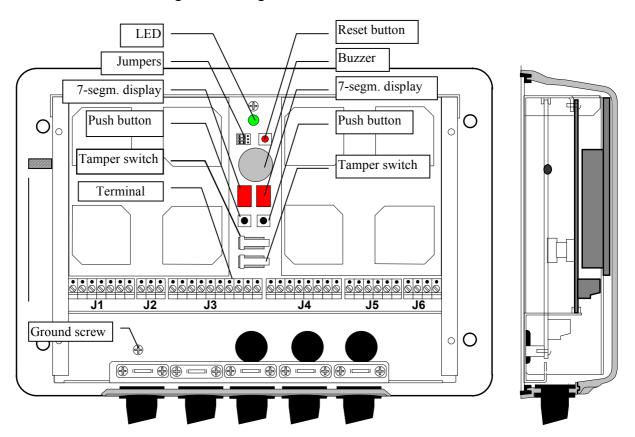
Connections to the Communicator are made using the terminal blocks J1 - J6.
