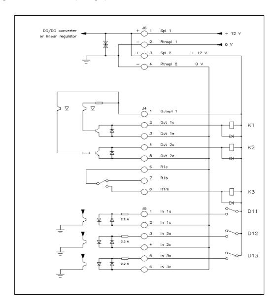
Optocoupler inputs: ON = from 2.4 to 30 VDC OFF = from 0.0 to 0.2 VDC
