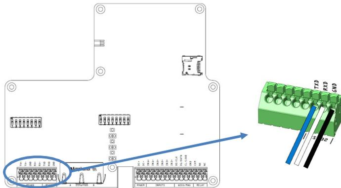
Figure 12 RS232 connection, overview and detail
