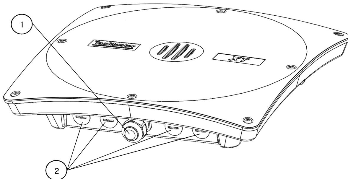
**Figure 3 Cable connections for XT-1 (Pos. 1 is M20 cable gland, Pos. 2 is M16 blind stops)**
