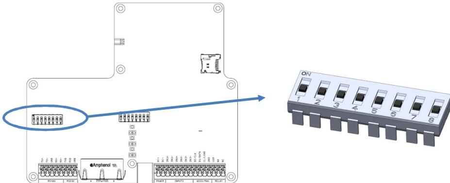
Figure 20 DIP SW S301, overview and detail
