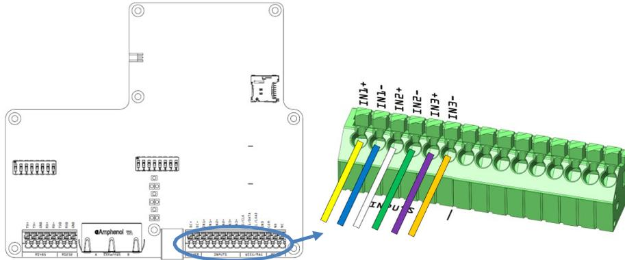
Figure 16 Input connections, overview and detail
