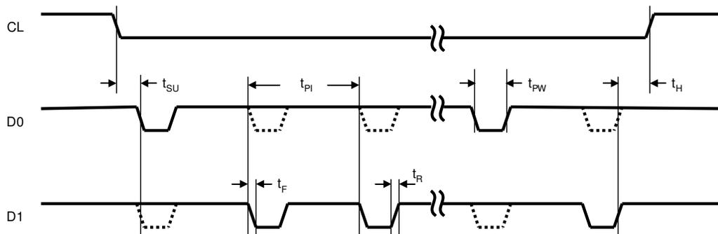
Figure 9 Wiegand timing diagram
