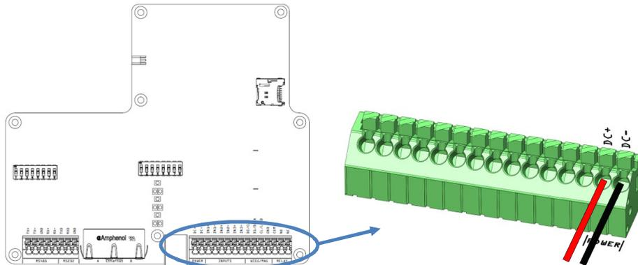
**Figure 7 Power supply connection, overview and detail**
