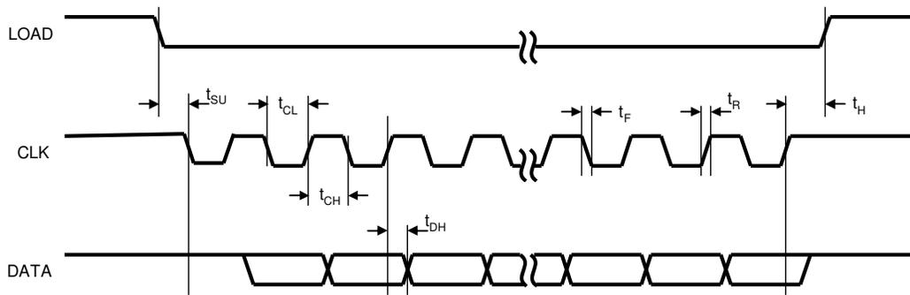
Figure 10 Magstripe timing diagram
