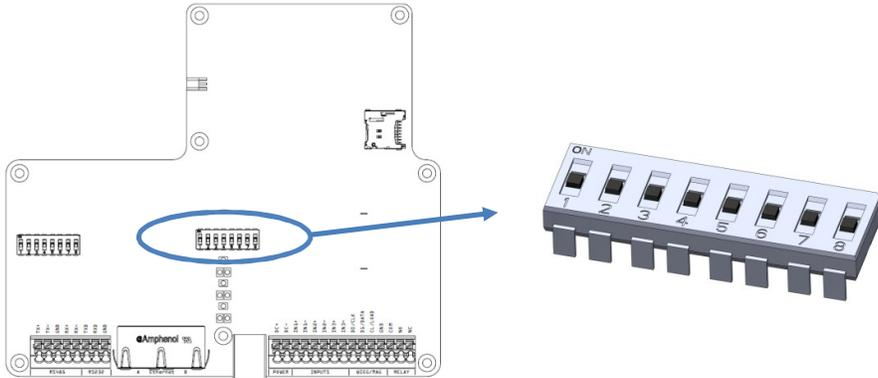
Figure 19 DIP SW S101, overview and detail
