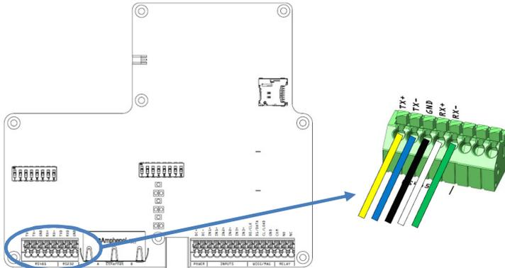
Figure 13 RS485 connection, overview and detail
