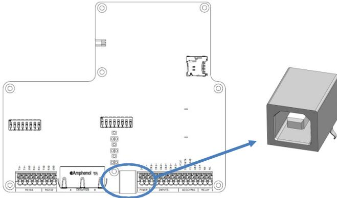
Figure 15 USB connection, overview and detail
