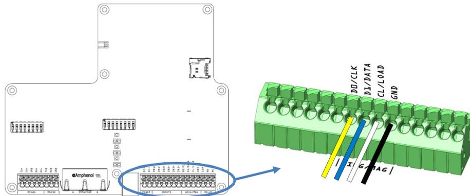
Figure 8 Wiegand connection, overview and detail
