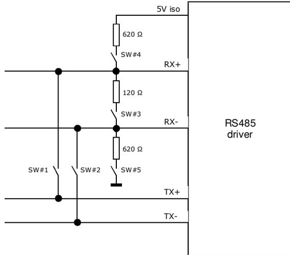
Figure 14 RS485 DIP switch configuration options
