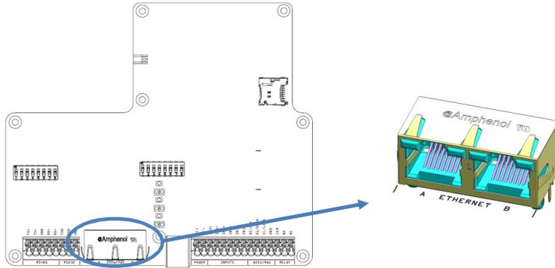
Figure 11 Ethernet connection, overview and detail
