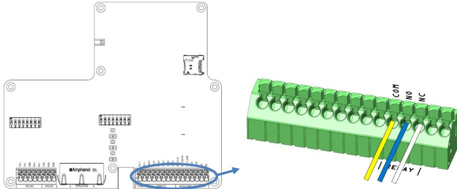
Figure 18 Relay connections, overview and detail
