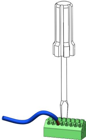
**Figure 6 Connection with easy-to-use spring cage terminal**
