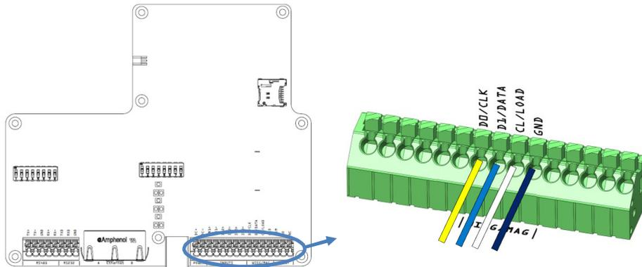
Figure 17 Output connections, overview and detail
