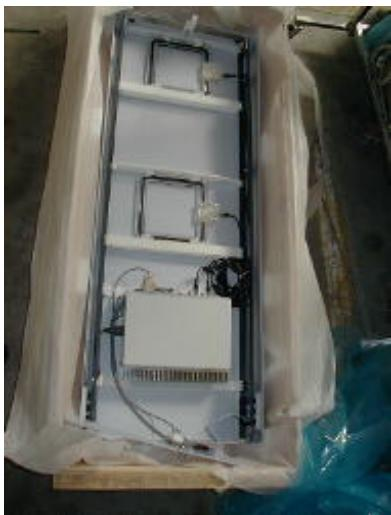
The station is composed of a TAG reader, one or several antennas matched and tuned during manufacturing test, a tallies and a hooding closed by back panels.
