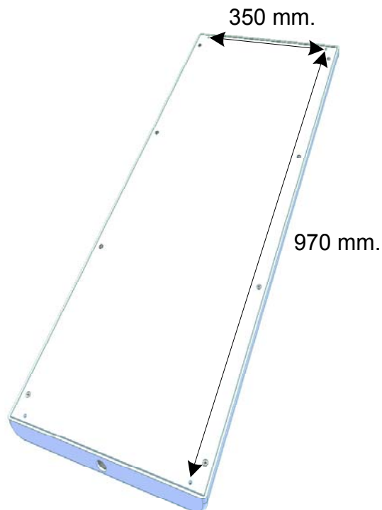
Figure 8: Conveyor Antenna Mechanical Diagram (Mounting Hole Dimensions)
