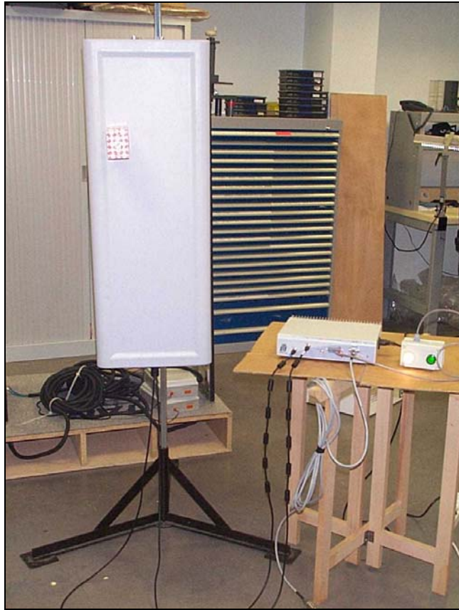
Figure 2: Full Conveyor Antenna System with the TR-L100 Reader and Signal Box
