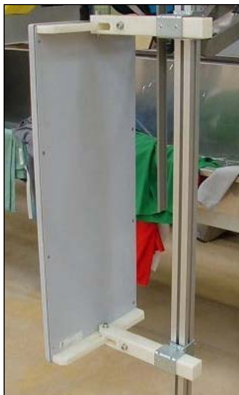
Figure 5: Mounting Brackets on Conveyor Antenna
