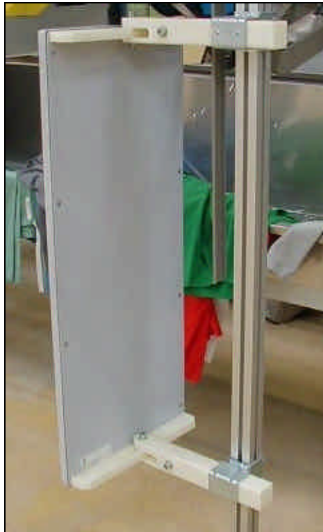
Figure 5: Mounting Brackets on Conveyor Antenna
