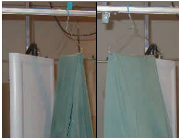
Figure 6: Conveyor Antenna used as a Guide
