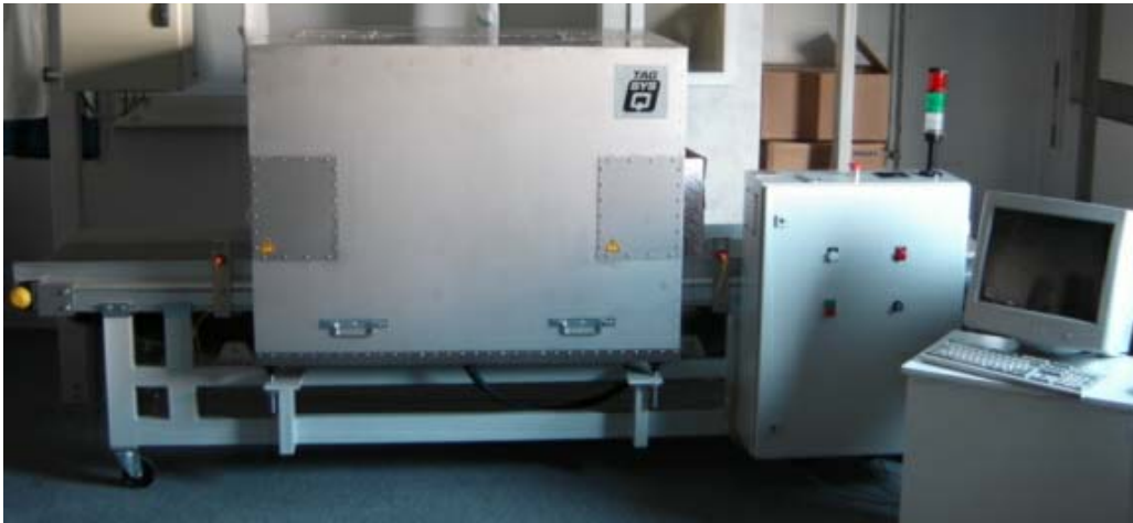
Figure 1 : Conveyor Tunnel Reader
