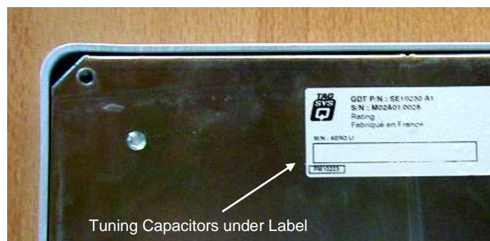
Figure 6: Position of the Tuning Capacitor on L-SA4 SHD Antenna
