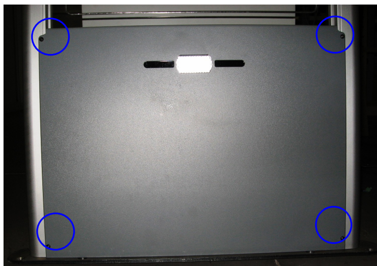
Figure 11: L-SP3 Clear Bottom Plastic Cover (4 screws)
