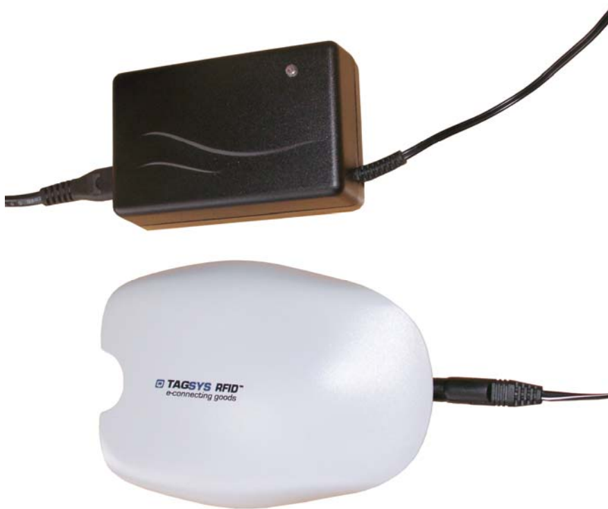
Figure 3: Connecting the battery charger
