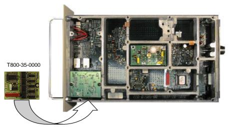
The T800-37-0000 fits inside of a T837-20-102x paging exciter. Installation is as simple as connecting the supplied ribbon cable to the paging exciter and selecting the required delay and data polarity using solder links.
