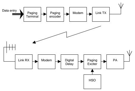
At the remote end, a T855 receiver is used to receive the signal from the central transmitter. This is then decoded by the T800-37-0000 modem board, which also adds the required amount of delay to the signal. The T801-20-0000 is used to generate the reference frequency, with the required offset. The T837-20-1021 then takes all of this to make the paging signal, which is fed to the PA and antenna equipment. And with any luck the subscriber has their pager turned on and receives the message.
