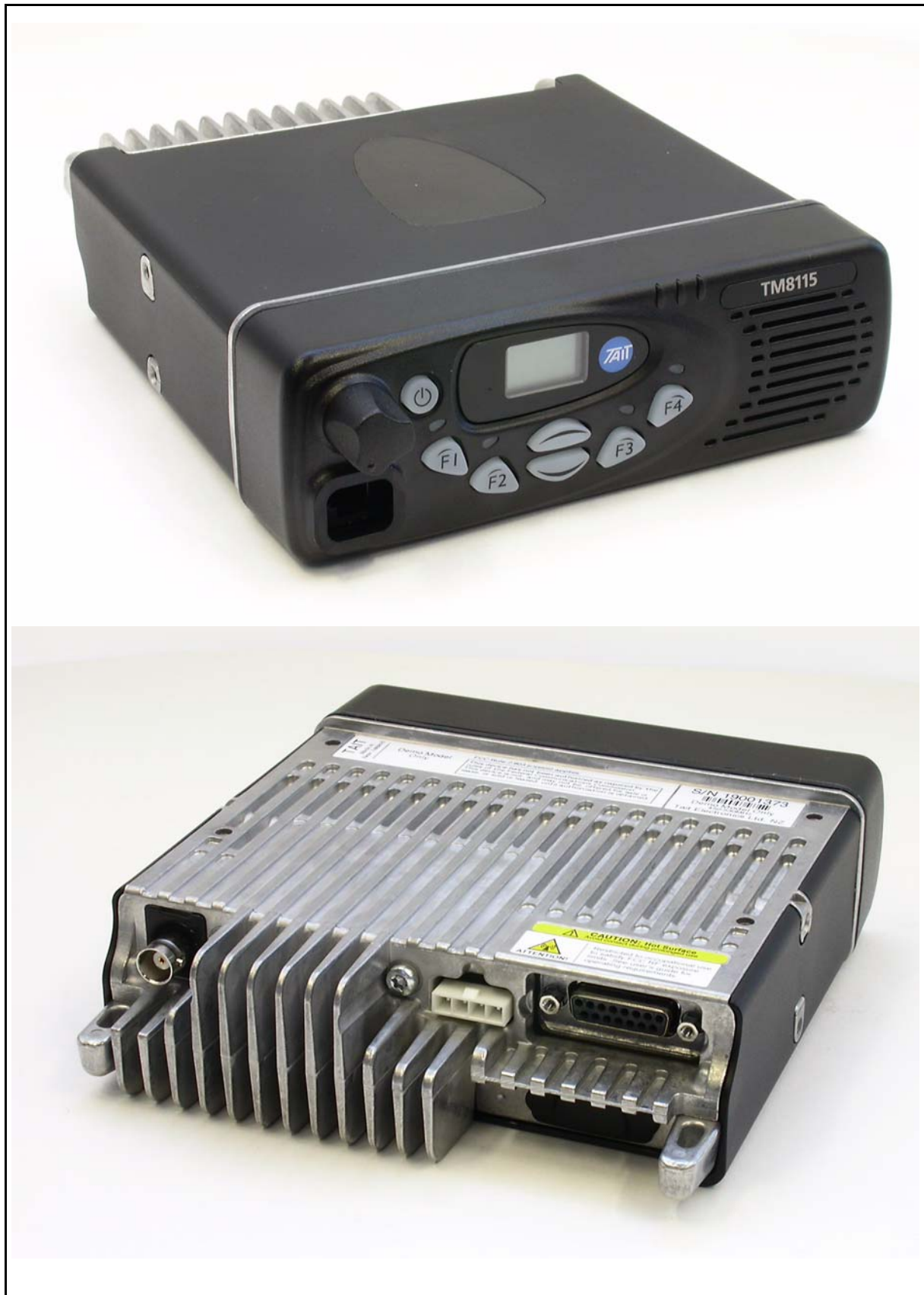
Figure 1.1 Illustrations of the TM8115 mobile radio showing both the front and rear
