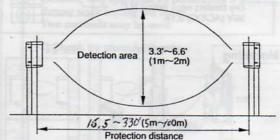
The protection distance should be between 3.3ft. (1m) and
