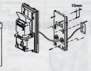
\*The grommet is compatible with a wire of  $\phi$  0.12" ( $\phi$  3mm) to  $\phi$  0.24" ( $\phi$  6mm) outer diameter.
