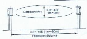
The protection distance should be between 3.3ft. (1m) and 165ft. (50m).
