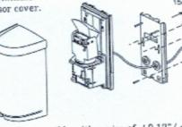
\*The grommet is compatible with a wire of \$0.12" (\$3mm) to \$0.24" (\$6mm) outer dia.
