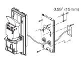
\*The grommet is compatible with a wire of  $\phi$  0.12" ( $\phi$  3mm) to  $\phi$  0.24" ( $\phi$  6mm) outer diameter.
