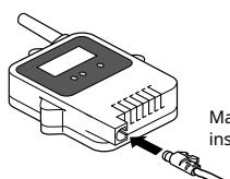
Make sure that the module is completely inserted until you hear a "click" sound.
