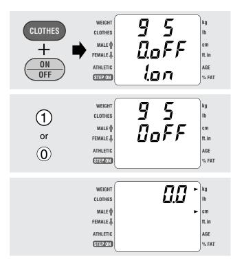
1. Press the CLOTHES key while holding down the ON key.
