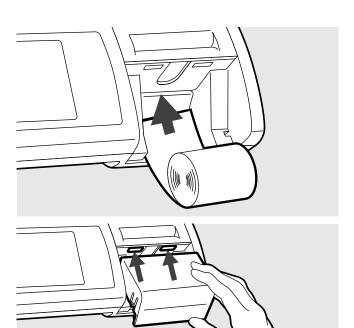
4. Insert the printer paper into the slit.
