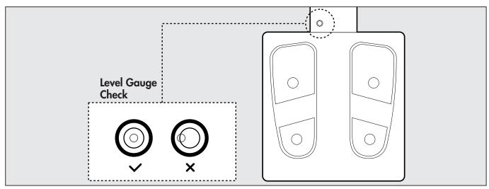
For accurate measurement, place the Weighing Platform on as flat a surface as possible and adjust the level with the adjustable feet so the bubble in the level gauge is in the center of the frame.
