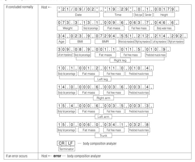
After measurement has finished, all necessary items of data and tare weight are cleared, and the unit waits for further commands.
