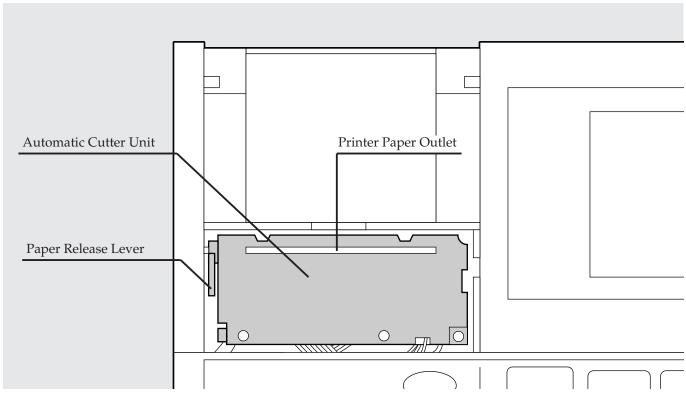
\* This is a picture of the Control Box without the Printer Dispenser Cover and the Printer Cover, looking down from above.
