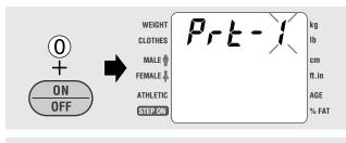
1. While holding down the [0] key, press the [ ON OFF ] key.
