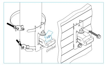
**Step 4.** Hang unit on gimbal, hooking inner hex/flange bolt into groove.
