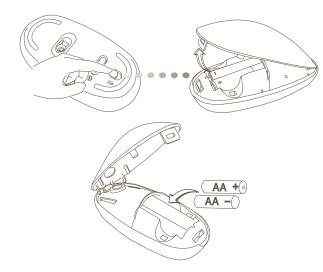
• Insert the batteries, making sure that the positive (+) and negative (-) ends of each battery match the polarity indicators inside the battery compartment.
