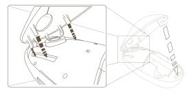
• Turn on the mouse by sliding the on/off switch on the bottom to the "on" position.
