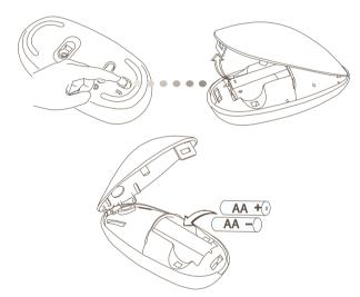
• Insert the batteries, making sure that the positive (+) and negative (-) ends of each battery match the polarity indicators inside the battery compartment.
