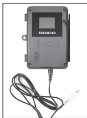
Cable from "AV Out"
