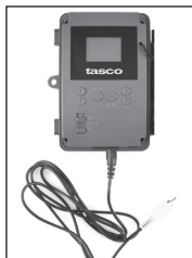
Cable from "AV Out"
