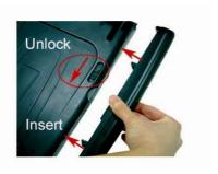
Unlock battery switch by pushing it downward.
