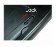
Release battery switch to lock it.
