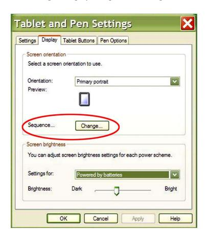
The sequence occurs when you press the screen rotational button with your stylus OR when you select **Change Screen Orientation** from the **Change Tablet and Pen Settings**
