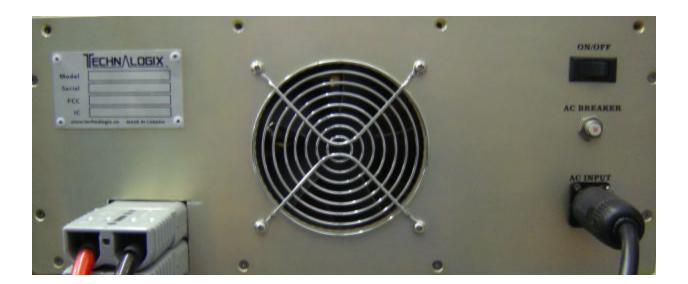
Tactile button to turn carriers on and off. To turn off, must be depressed for at least 2 seconds. Tied internally through DB9 connectors to all other POWER buttons.
