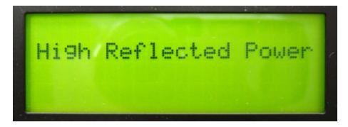
This message indicates that excessive reflected power has been detected at the output of the transmitter. Periodically, the amplifier will cycle on, and re-check for reflected power. If high reflected power continues, the transmitter will eventually shut down completely.
