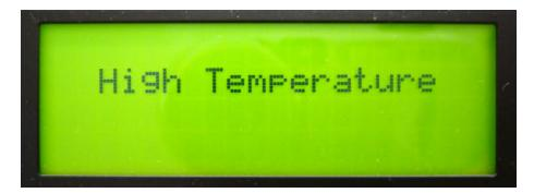
This message indicates that the transmitter is experiencing unsafe internal temperatures. Output power is reduced until a safe temperature is reached.
