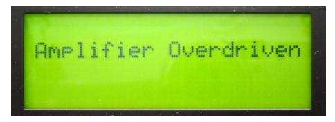
If you see this message, the system has been driven to a power level higher than it is rated for. This message will likely only appear momentarily, before the amplifier will add attenuation at its input to bring the output power to a safe level.
