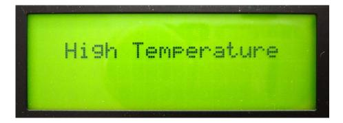
The control system monitors the temperature of a specific location of the heat sync. If this temperature exceeds a threshold the control system will turn the RF output level down until this temperature level is reached. The RF output level will automatically be brought back when it is safe to do so.
