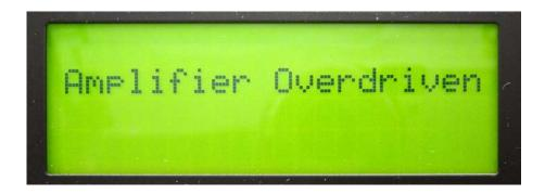
The Amplifier overdrive shutdown is set to 115%. If the Amplifier is being overdriven (the RF output level is too high) the control system will automatically attenuate the RF input signal to the PA. It will continue attenuating this signal until the RF output is below 115% total power.
