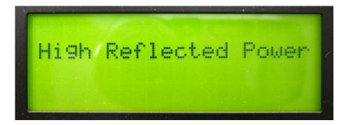
If Reflected Power has been detected at the output of the transmitter, the unit will shut down for 4 seconds. This occurs 5 times – If the fault is clear the PA enables itself. If the fault still exists after 5 times, the PA disables the carrier for 10 minutes and cycles until the fault clears. During the disable time (10 minutes) the unit will still alarm with a High Reflected message on the front panel.
