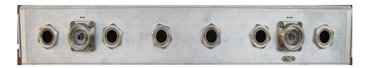
RF IN - RF inputs (500-watts each) from the power amplifier. N female connector, 50 ohm.
