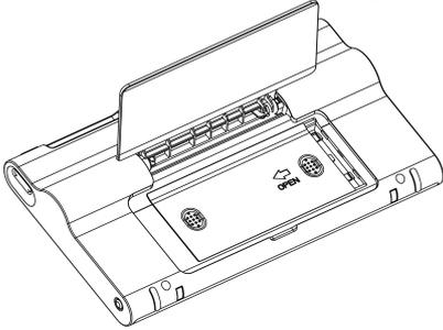
3. Plug the battery pack cord into the jack inside the compartment.
