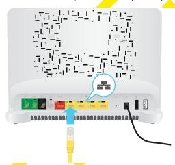
You can not use the red WAN port to connect to the local Ethernet network. The WAN port can only be used to connect your Technicolor Gateway to your broadband source.
