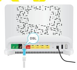
3 Plug the other end of the cable into the DSL/MODEM output port of your filter/splitter.
