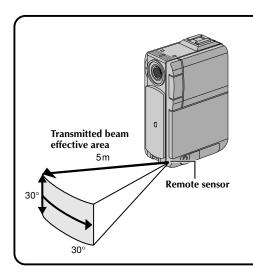
When using the remote control, be sure to point it at the remote sensor. The illustration shows the approximate transmitted beam effective area for indoor use.
