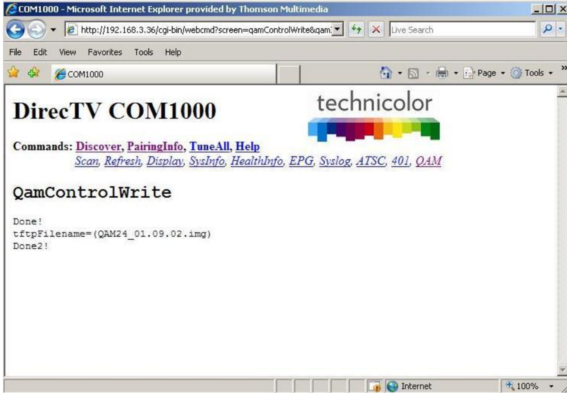
Figure 59 – QAM24 SW Upgrade Results
