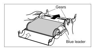
10 Close the covers of the cartridge by locking the four tabs.
