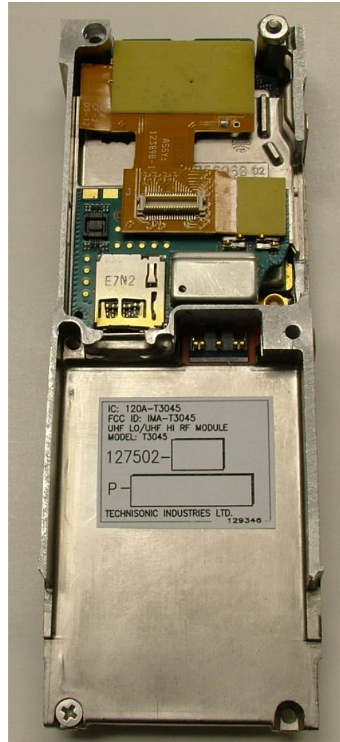
FIGURE 2 APX 7000 FCC ID (Left), Right T3045 Module with new FCC ID applied
