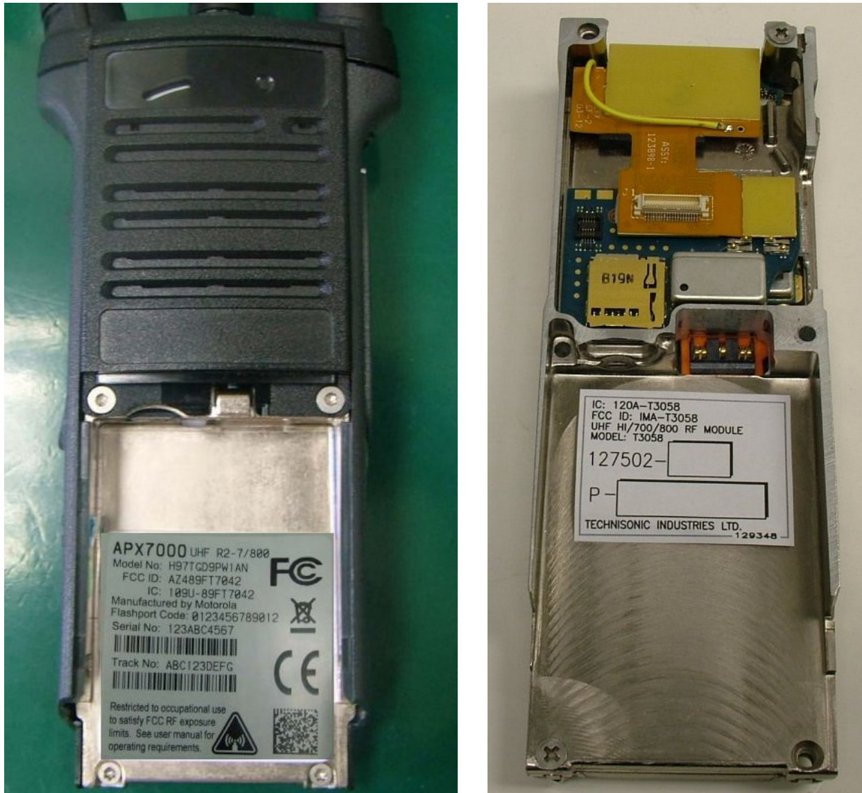
FIGURE 2: APX 7000 FCC ID (Left), Right T3058 Module with new FCC ID applied
