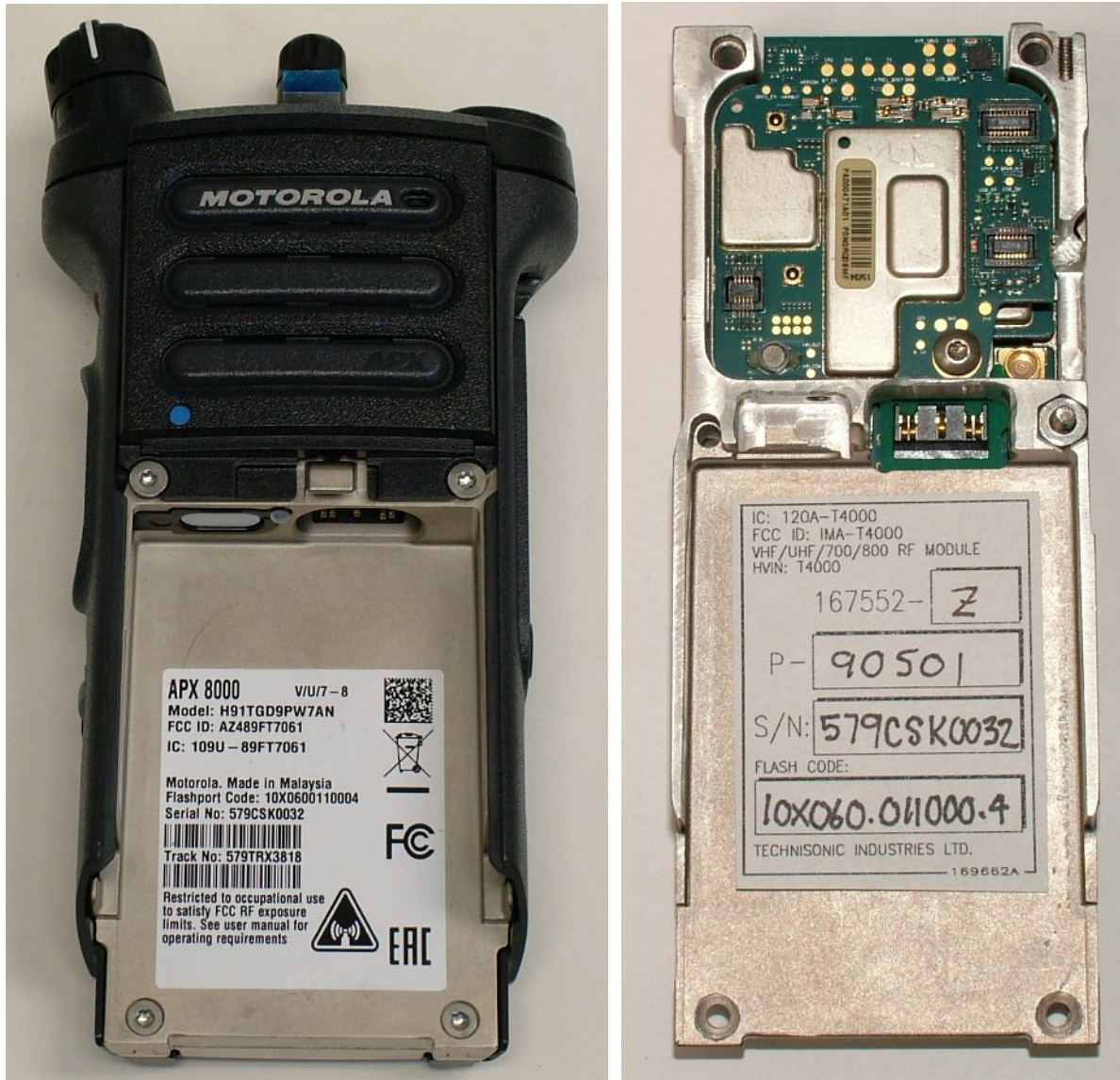
FIGURE 2: APX 8000 FCC ID (Left), Right T4000 Module with new FCC ID applied
