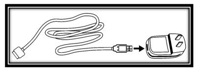
2. Hold the Tablet so that the screen side is facing you and the recharge port is aiming downwards. Make sure the tactile HumanWare logo on the recharge cable is facing you (1). Carefully connect the cable to the recharge port and plug it to an outlet.
