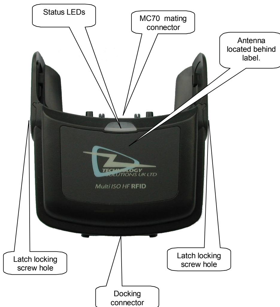
Figure 1: The parts of the RFID 1059
