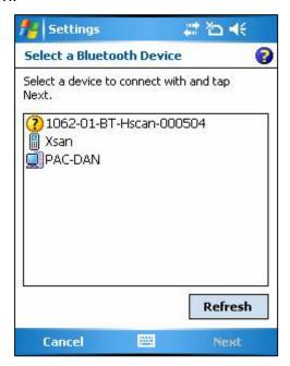
By default the Handscanner name corresponds to the serial number printed on the side of the unit. In this case it is'1062-01-BT-Hscan-000504'. Tap on the Handscanner and then on 'Next'.
