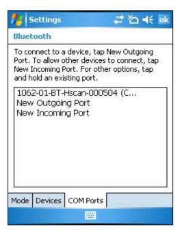
Any application which opens this virtual comm. port (COM 4 in this example) will be connected to the Handscanner.
