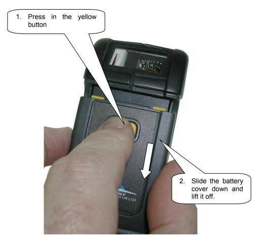
The battery can then be lifted out and replaced. Refit the cover by sliding it back up until the button clicks in place.
