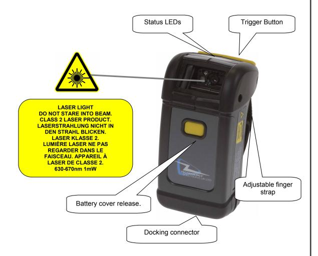
The status LEDs on the top of the Handscanner provide an indication of the operating status of the unit.
