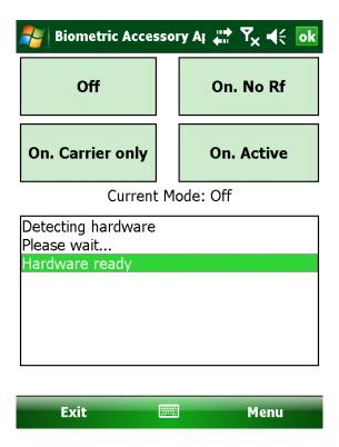
NOTE: For the accessory to change to some modes an RFID card must be present in the field. A card has been provided for this purpose. It is only required to change the mode. The current mode is displayed on the screen. Any errors are displayed in the list view below the buttons.
