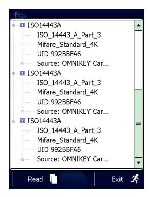
As the application is launched a splash screen is displayed while the hardware is detected. Once detected it switches to the main screen and starts the RFID reader. While a card is present it is output to the screen. If no card is present for a period longer than an idle timeout (30s) the reader powers off. The read button will restart the process. Exit will exit the application.
