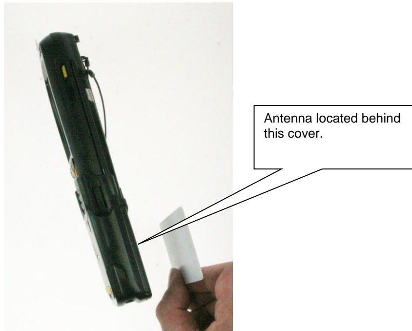
Figure 6: Antenna location and read direction
