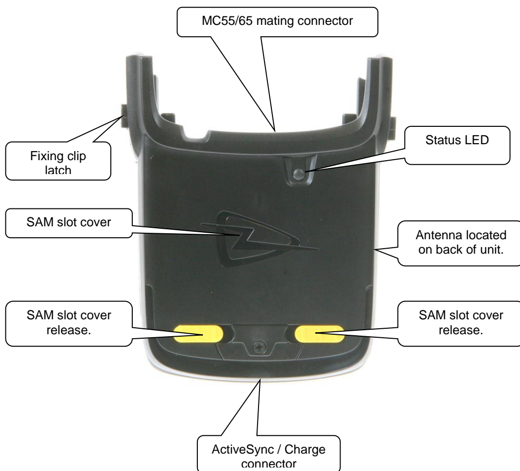
Figure 1: Parts of the 1117 HF Reader
