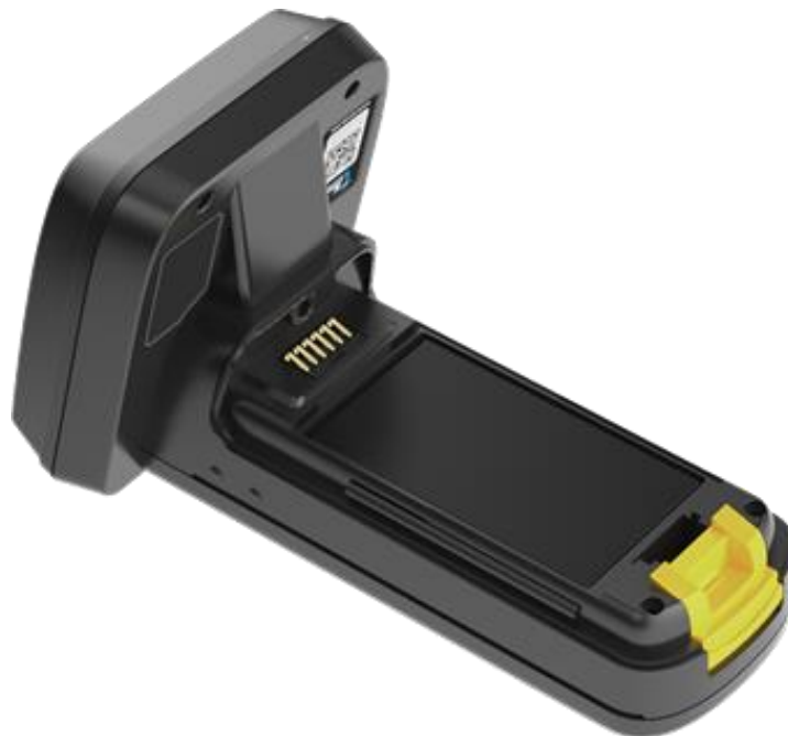
Figure 8: Battery in position
