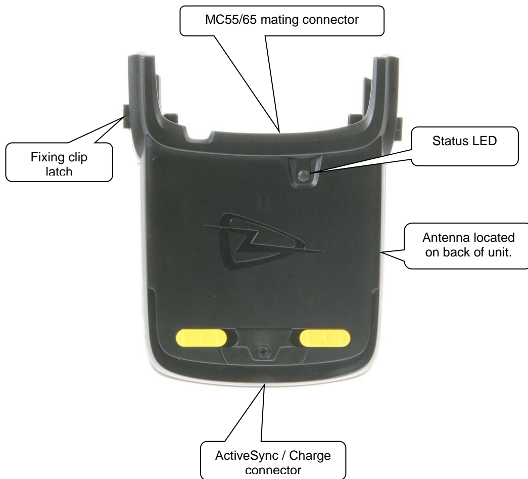
Figure 1: Parts of the 1134 LF Reader
