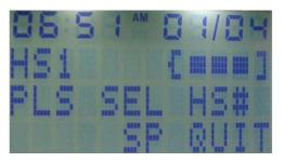
Step3. User may press Handset number for handset to handset intercom operation. For example "4", it means intercom with handset 4.
