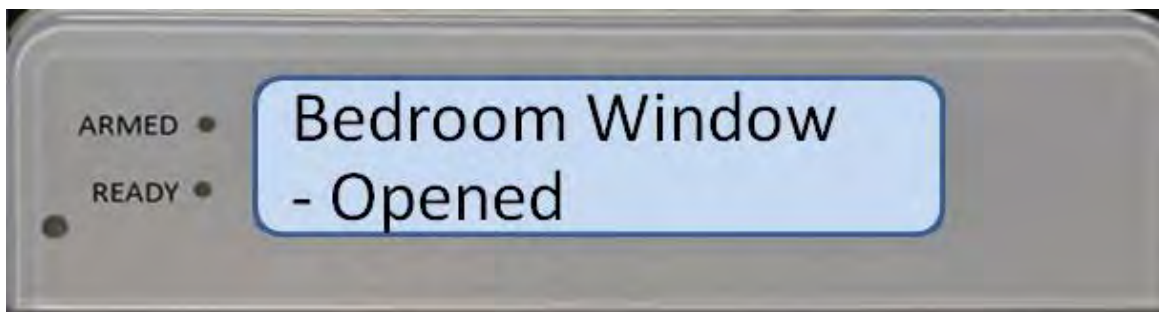
Figure 90: Keypad – Example: Bedroom Window Open
