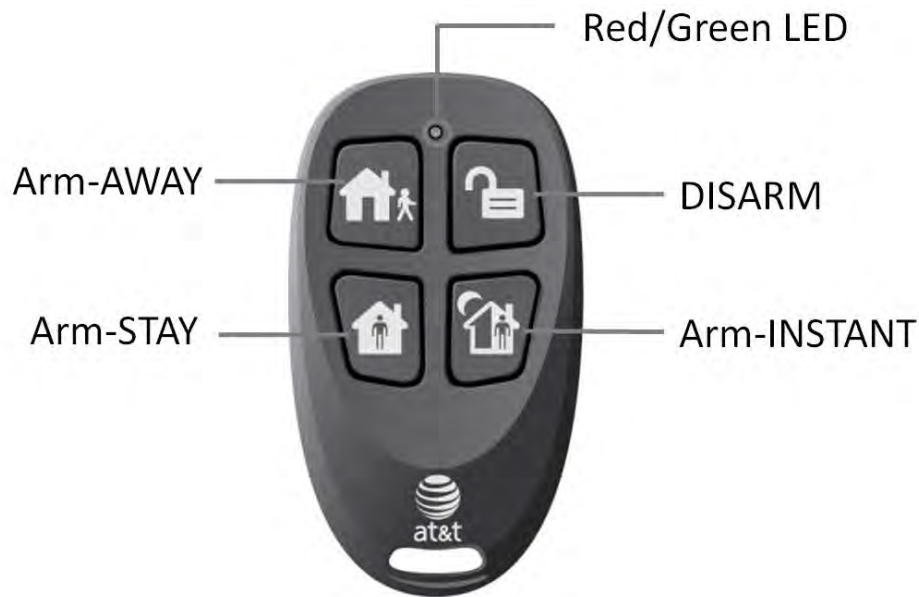
Figure 48: Keychain Remote (Model SW-ATT-FOB2)
