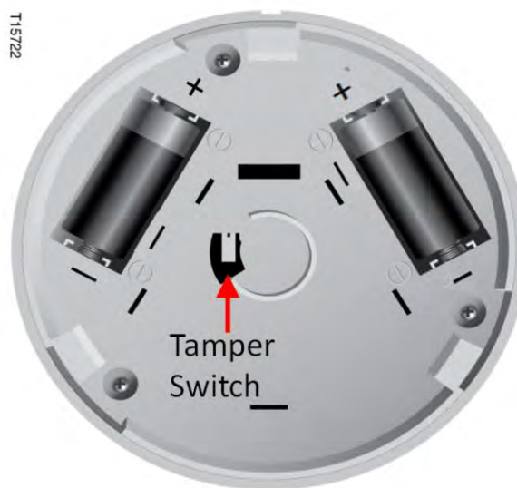
Figure 73: Installing/Replacing the Glass Break Sensor (Model SW-ATT-GB) Batteries
