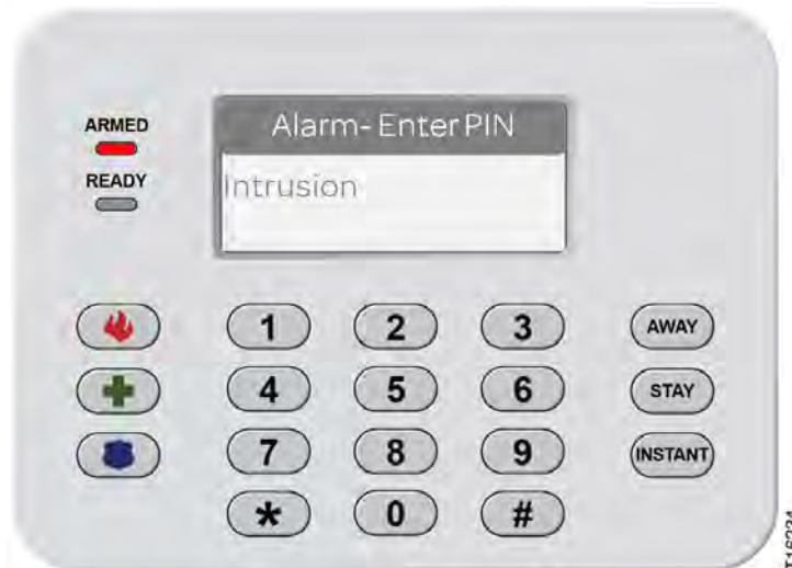
Figure 108: Keypad (Model SR-KPD02)—Alarm- Enter PIN (Intrusion)
