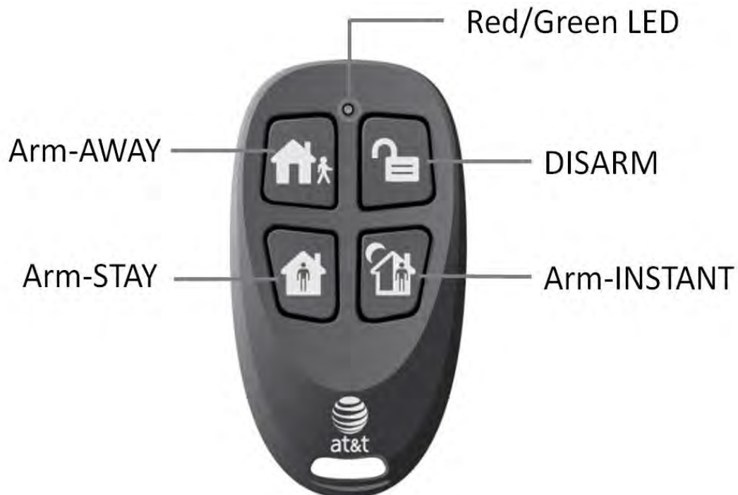
Figure 120: 915 MHz Two-Way Keychain Remote (Model SW-ATT-FOB2)
