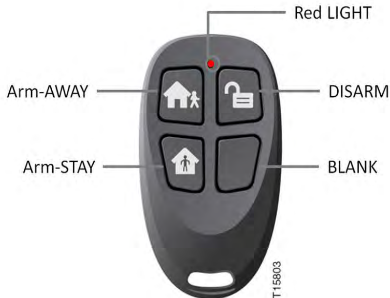
Figure 119: 433 MHz One-Way Keychain Remote (Model SW-ATT-FOB) ( SW-ATT-FOB)
