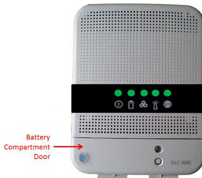
Figure 41: Battery Compartment—Front Panel
