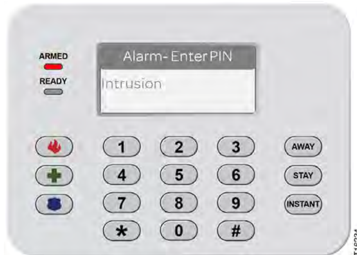
Figure 108: Keypad (Model SR-KPD02)—Alarm- Enter PIN (Intrusion)
