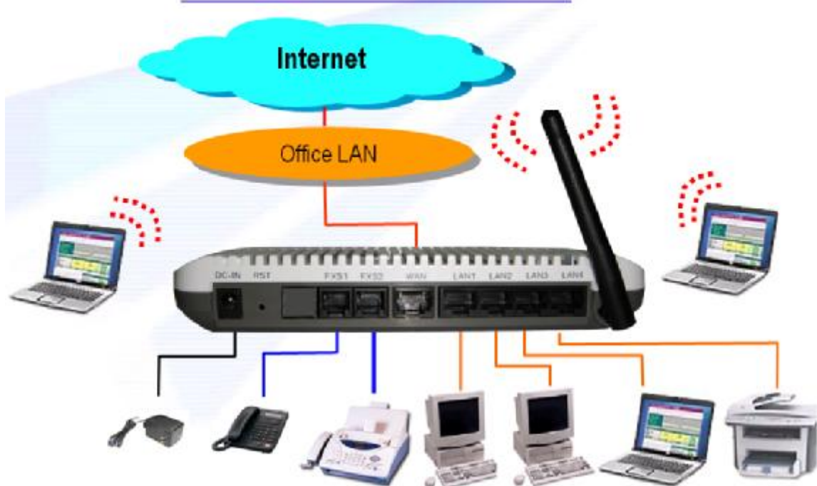
Figure 4.3 The Connection of 2/1-port FXS ATA WiFi-Router at Office
